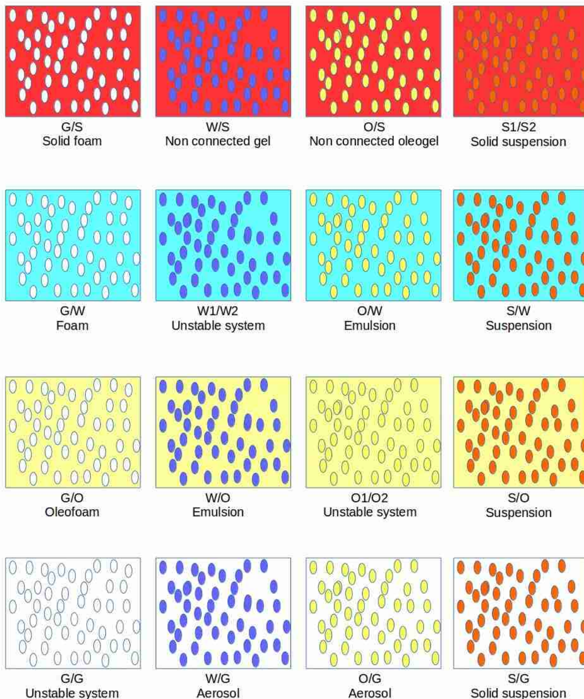
Figure 1. The simplest disperse systems for which one phase is randomly dispersed in another phase. The operator “/” indicates the random dispersion. The letters G, O, S, and W respectively stand for gas, oil, solid and water. Under each system, the traditional name is given. Formula such as W_1/W_2 or O_1/O_2 are meaningless, because they can be reduced to W or O respectively, and they are no disperse systems.
